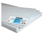
Polyester fibre sheet for decoupling and soundproofing reduction under bonded parguet indoors also appropriate for applying a levelling layer before bonding textile and elastic flooring.
