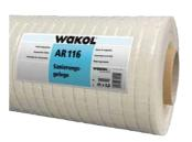
Fibreglass strips laminated on backing fleece for the usage on cracks and joints in subfloors without counter movements up to maximum 5 mm width instead of force-fit connection, screed damages and mixed subfloors indoors.
