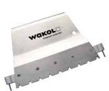
Special notch to form a moisture barrier on unheated cement screeds up to 4 CM% resp. 85 % corresponding relative humidity for laying parquets (all types of parquets with tongue and groove joint) with WAKOL MS 262 Parquet Adhesive, firm-elastic, WAKOL MS 260 Parquet Adhesive, firm-elastic, WAKOL MS 230 Parquet Adhesive, elastic or WAKOL MS 228 Ready-to-lay Parquet Adhesive, elastic.
